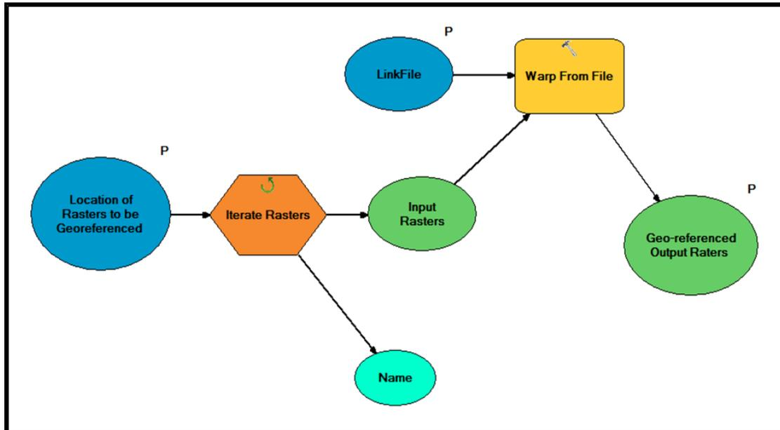
Figure 6: Model for Batch Geo-Referencing
