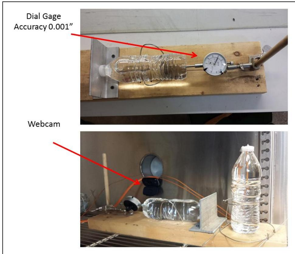
**Figure 5:** Bulging Experiment Setup
