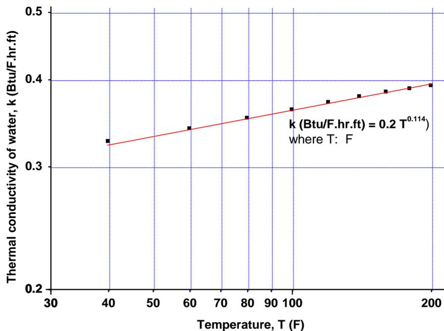
Figure 1: Thermal Conductivity of Water as a Function of Temperature
