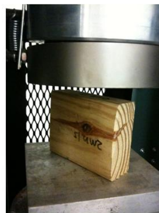
Compression Test Load applied slowly
