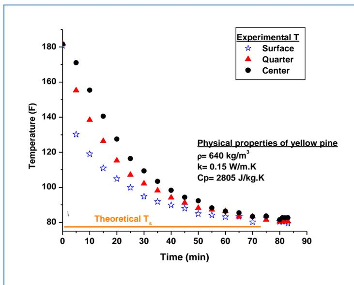
Figure 9: Comparison of Experimental and Theoretical Surface Temperatures
