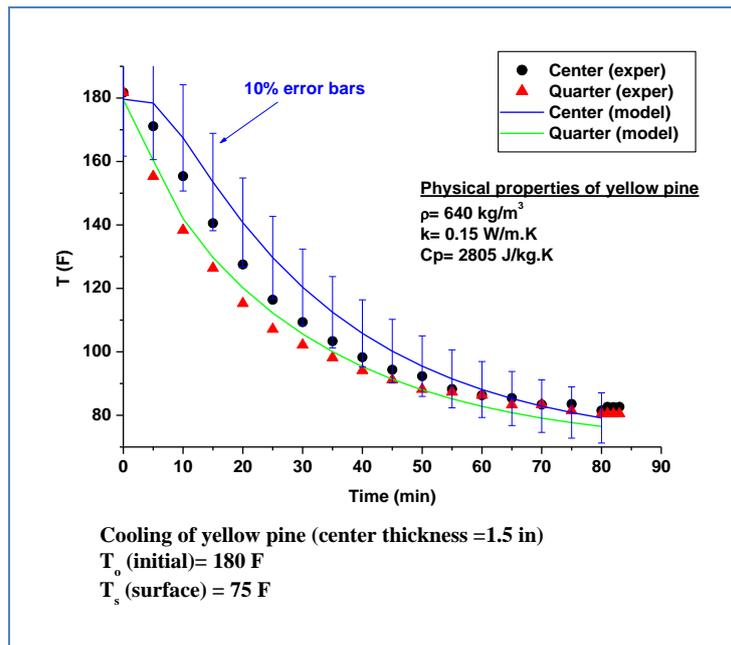
Figure 8: Comparison of Temperature Profiles (Experimental vs. Model)
