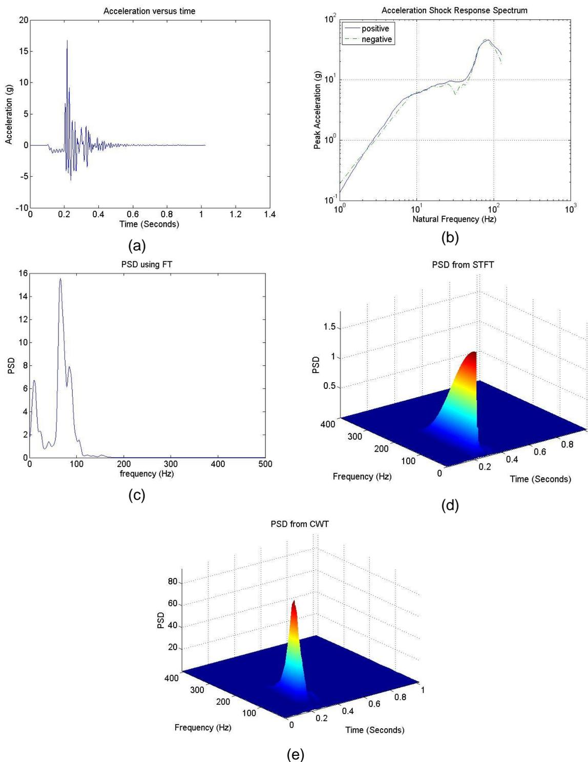
**Figure 3:** Data Measurement and Analysis for 2 Inch Pallet Drop Measured in the Direction of the Drop. Shock Acceleration versus Time Measurement (a), SRS (b), PSD from FT (c), PSD from STFT (d), and PSD from CWT (e)
