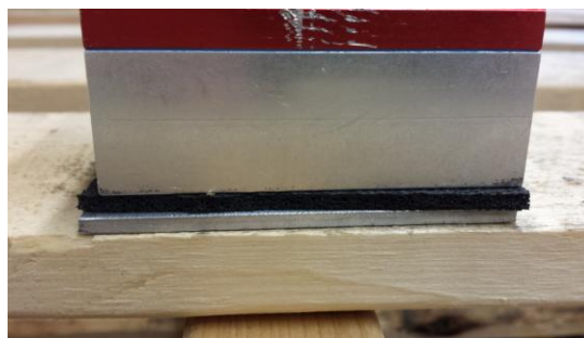
Figure 5: Aluminum Plate Placed on the Pallet Top Board with Cushion above (Case 4)
