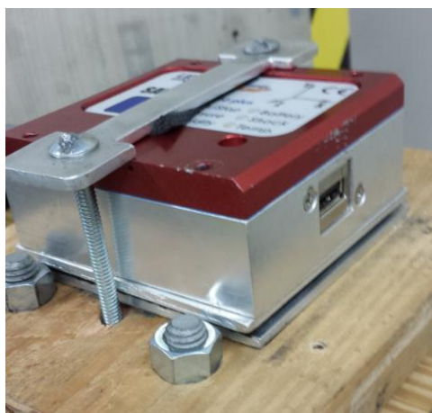
Figure 6: Anti-vibration Pad Placed Between Two Aluminum Plates (Case 5)
