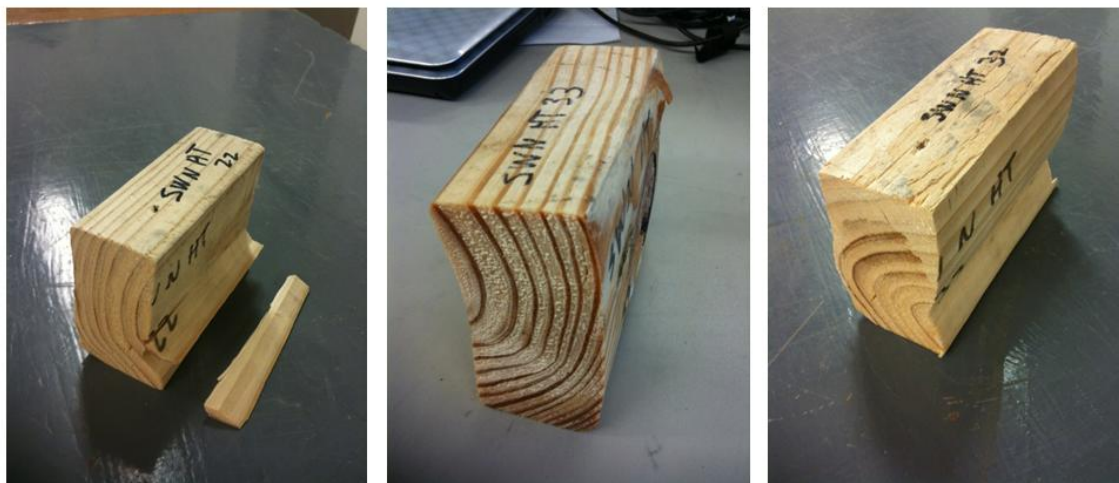
Figure 2: Failures of Specimens with Different Grain Orientations
